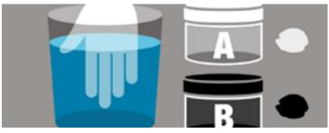
2. Using wet gloves, take one Part A and one Part B of equal size.
