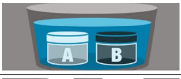
1. In cold conditions immerse tubs A and B in warm water for 30 minutes. This will loosen the product for ease of application.
