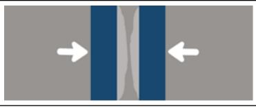
4. Apply a small amount to each of the intended substrates and press firmly together.
