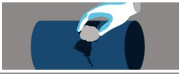
5. With the aid of wet gloves, apply and mould to required profile.
